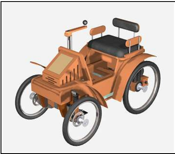
Figure 8, Bonnet, dash panel, seat rests & mudguards added.
