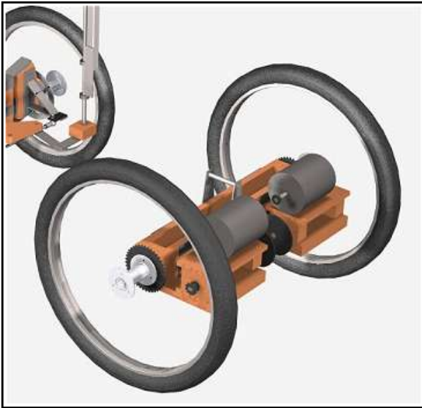
Figure 4, Rear wheel electric drives.
