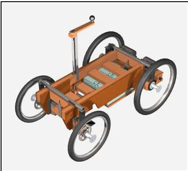
Figure 6, Showing subframe cross bracing and battery position.
